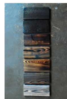
Charred Accoya Cladding
