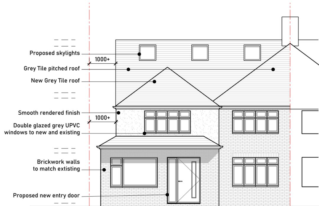
**Proposed Front/South Elevation**
